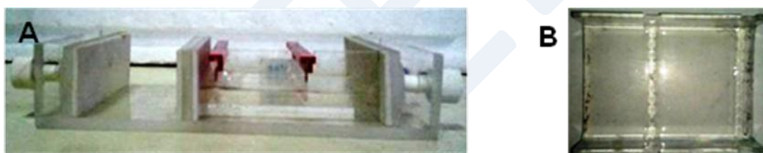
Figure 1: A. Agarose gel casting unit. B. Solidified agarose gel.
